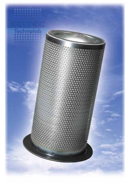
The standard conventional oil separator is the original design for the removal of oil aerosols from the compressed air stream. This element design consists of a specific amount of a uniform grade of borosilicate glass fibers, "wrapped" onto a support tube. When properly sized to the cfm/m3/ min flowrate and corresponding operating pressure of the machine, this element will provide consistent performance according to the following data:
